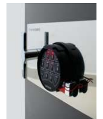
Battery case / keypad top lit LED
